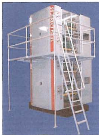
To put process color on each side of a web, stacked S4 units use one impression cylinder (above) and a Tech Express tower uses four.
